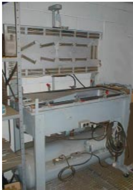
Figure 2 - Vacuum Forming Machine
